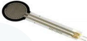
Figure 8: Force Sensitive Resistor
